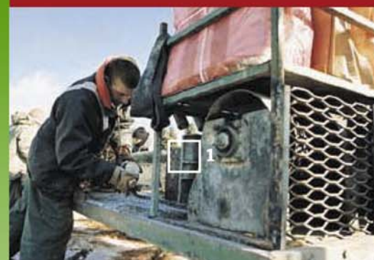
The emergency stop barrier (1) allows the worker to turn the winch's drive mechanism off by opening the door. The barrier must be closed before the mechanism can be reactivated.
