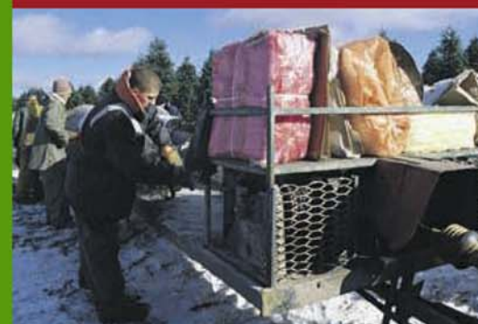
Rear view of the wrapper. The power takeoff and the screen protecting access to the winch are clearly visible. The winch has a quick-response stopping mechanism for emergencies.
